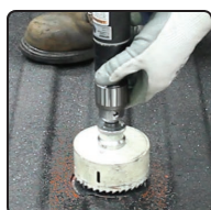
Use the pilot hole for error-free drilling
