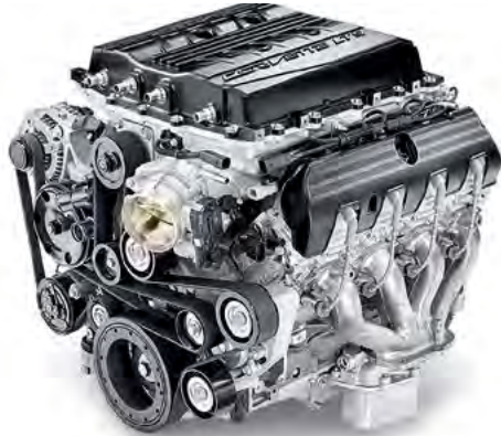
6.2L LT5 SUPERCHARGED V8 (STANDARD ON ZR1)
