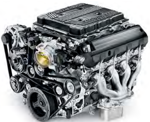
6.2L LT4 SUPERCHARGED V8 (STANDARD ON Z06)
