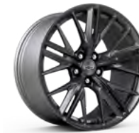
20" x 10" front and 20" x 11" rear 10-split-spoke Dark Graphite-painted forged-aluminum (RTQ) Standard on ZL1
