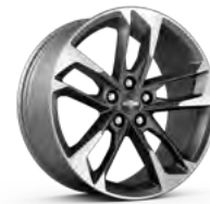
20" x 8.5" front and 20" x 9.5" rear blade-design aluminum (56Y) 3 Available on 2SS
