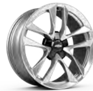
20" x 8.5" front and 20" x 9.5" rear 5-split-spoke polished forged-aluminum with Black Star centre cap (57W) Available on SS
