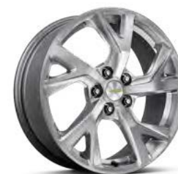
18" machined-face aluminum wheels with painted pockets (RV6) Available on LT with 1.5L engine Included on LT with 2.0L engine
