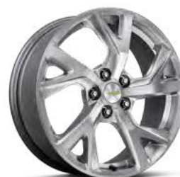
18" machined-face aluminum wheels with painted pockets (RV6)
