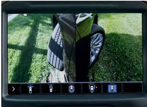
Front Side View Shows the position of the front tires when parking and during tight manoeuvres.
