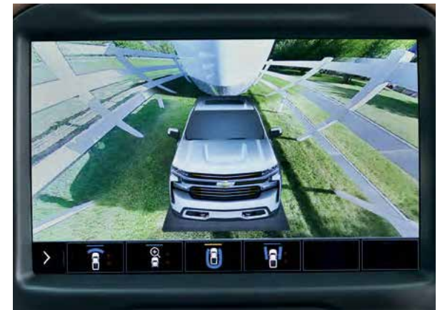
Bowl View Provides a rear-facing 3-D surround view, useful for low-speed backing manoeuvres.
