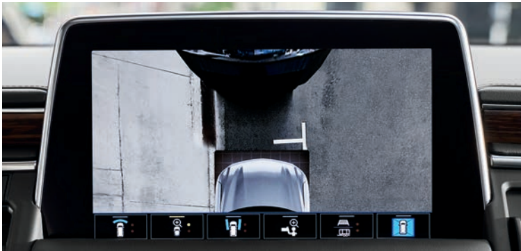
Front Top-Down View A top-down view of the hood, bumper and front tires for tight maneuvers in parking lots or along curbs.
